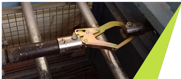
Static Load Testing of Rebar Hook
