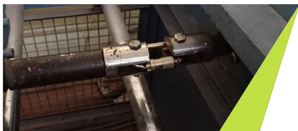
Static Load Testing of Karabiner
