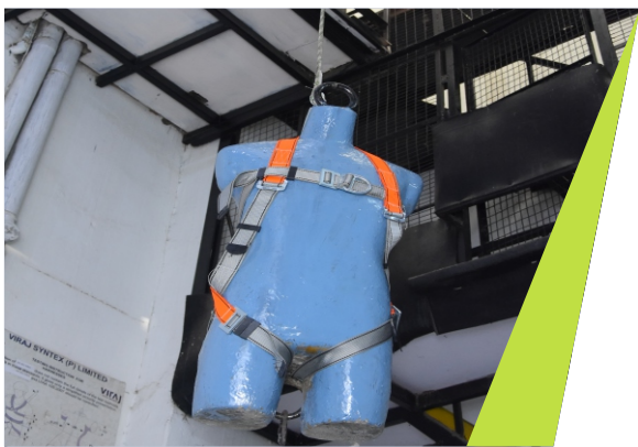
Dynamic Load Testing
