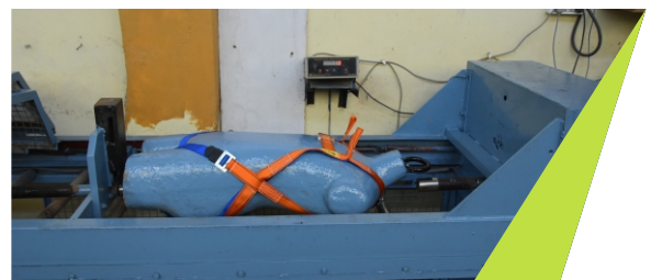
Static Harness Load Testing
